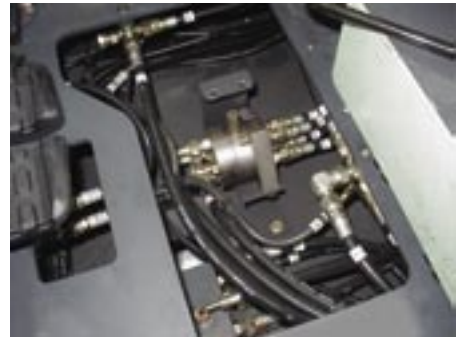
Control Pattern Selector Valve - located in the floor of the cab
