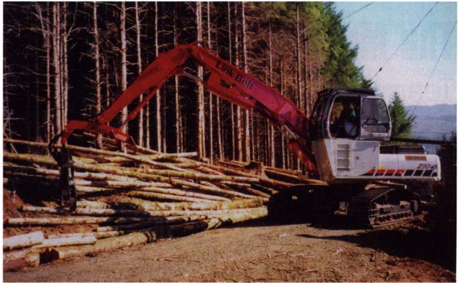
Long, straight stems make stroke boom delimiting the option of choice in many of the Northwest's second and third growth forests like those in the background.
