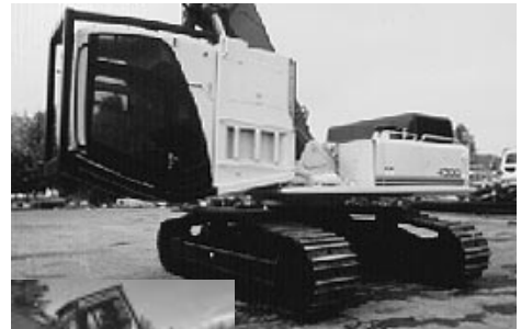
Cab completely tilts forward for ease of transportation and servicing. Hydraulically controlled from side of upper.
