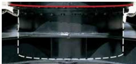
Built into the "X" style carbody is the turntable bearing "tub" which extends down through the top plate and is welded to the bottom of the carbody as well as the top for increased strength and durability
