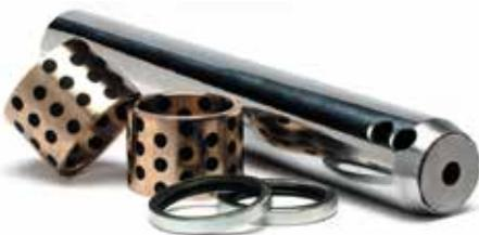
Chrome plated pins with brass bushings throughout the entire attachment (except bucket) make a durable and long lasting connection at these high stress points. This also makes it possible to extend the lubrication interval on this type of pin to once every 6 months or 1,000 hours of operation, whichever comes first.
